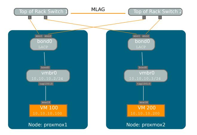
Another possibility it to use the bond directly as bridge port. This can be used to make the guest network fault-tolerant.
