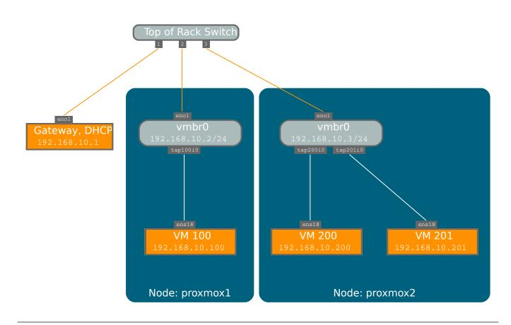
Bridges are like physical network switches implemented in software. All VMs can share a single bridge, or you can create multiple bridges to separate network domains. Each host can have up to 4094 bridges.
