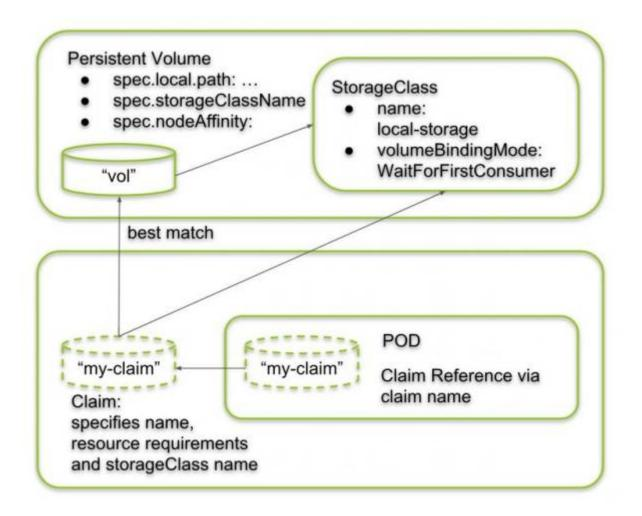
Once a POD is created that references the volume claim by name, a "best match" choice is performed under the restriction that the storage class name matches as well.
